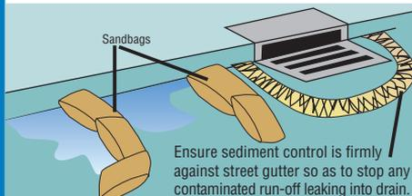
Ensure sediment control is firmly against street gutter so as to stop any contaminated run-off leaking into drain.
