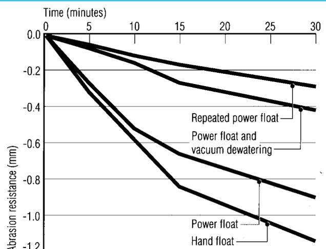
Figure 2 and Figure 3 illustrate the importance of the finishing process and curing. These graphs show that if a hard abrasion resistance surface is
