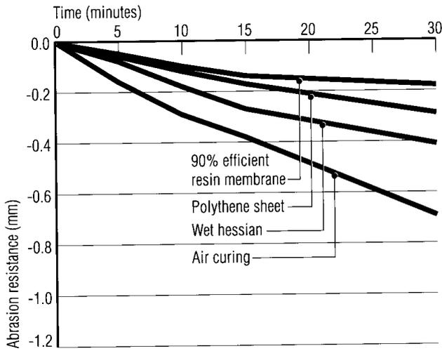
required, specify that repeated power trowelling is required and ensure curing is effective and occurs as early as possible. Be aware that hard steel trowelling will probably result in a crazed surface;
