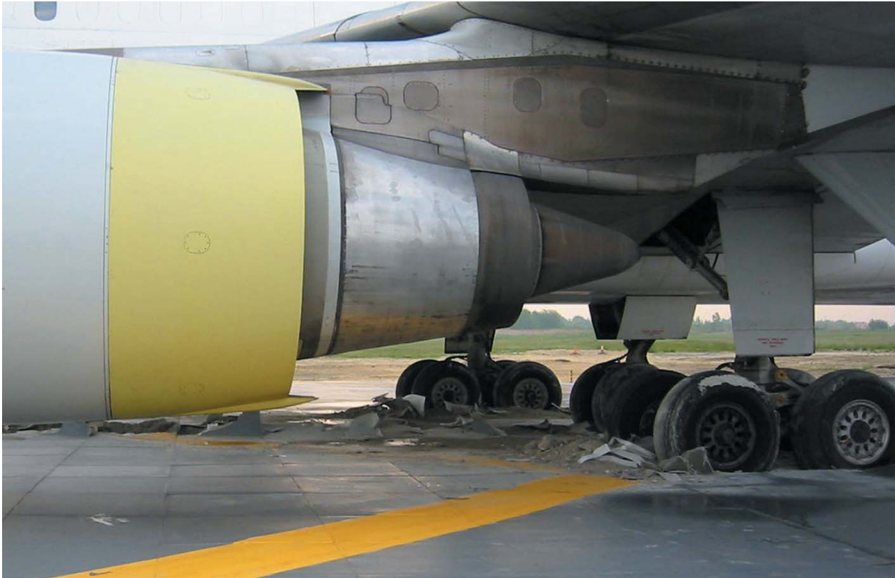
MD-11 cargo plane arrestment at JFK International, May 2003. Photo courtesy of the Port Authority of NY & NJ
