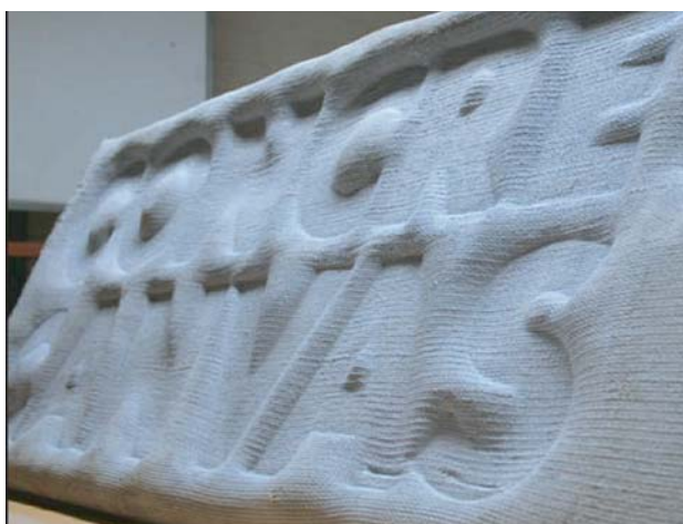
Concrete cloth is a ceramic-based material; it is flexible, can be cut using simple hand tools and will not burn.
