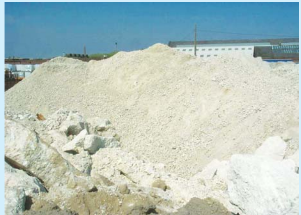
Recycled aggregate stockpile.
